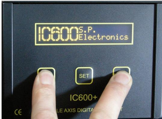
The "**ADVANCED CONFIGURATION**" is accessed by pressing and holding the "UNIT" and "MODE" buttons from the Firmware screen
