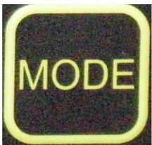
This button allows a change in the number of decimal places displayed it also allows the operator to re calibrate the IC600 if required.
