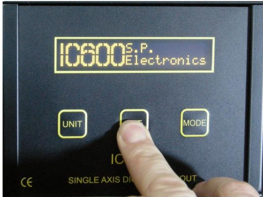
The "SIMPLE CONFIGURATION" mode is accessed by pressing and holding the "SET" button from the Firmware screen until "SIMPLE CONFIG" is displayed.
