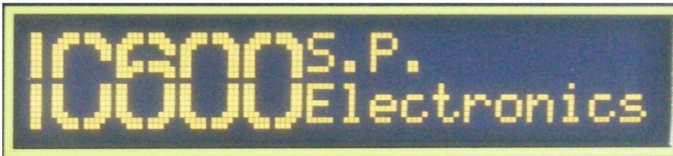
The "IC600 PLUS" will display the current position, this is the position that was stored at power off and will be correct assuming the gauge has not moved whilst the unit was switched off.
